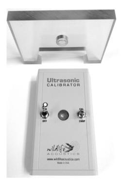
WARNING: In "Chirp" mode, the Ultrasonic Calibrator emits a 40khz signal at over 100dB SPL. Prolonged exposure to high intensity ultrasonic signals may cause permanent hearing loss at audible frequencies. Please do not place the Calibrator close to your ears!
