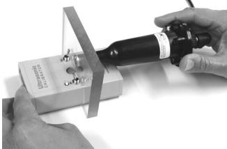
Insert the microphone until it rests against the smaller diameter of the adapter hole as shown below.
